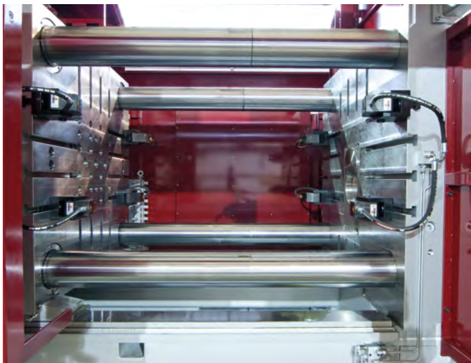
Piani in acciaio forgiato con riporto in Inox. Platens made of forged steel with stainless steel coating.
