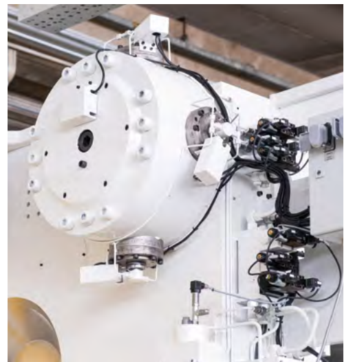
Sfilamento colonna superiore. Removal of upper tie bar.
