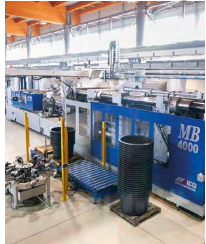
Pressa specifica per produzione di grandi contenitori Specific I.M.M. for production of very large vases Machine à Injecter spécifique pour production de grands vases
